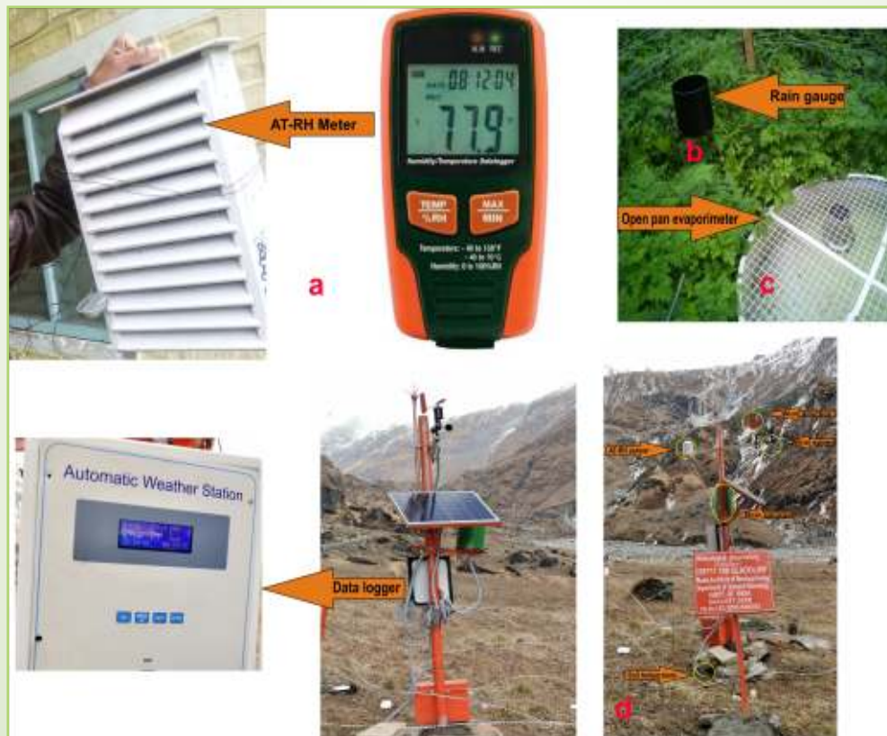
Fig. 51: (a-c) AT-RH meter, rain gauge and Evaporimeter installed at Dwali station. (Fig. d) meteorological Observatory/ AWS established at Kafni glacier zero point.
