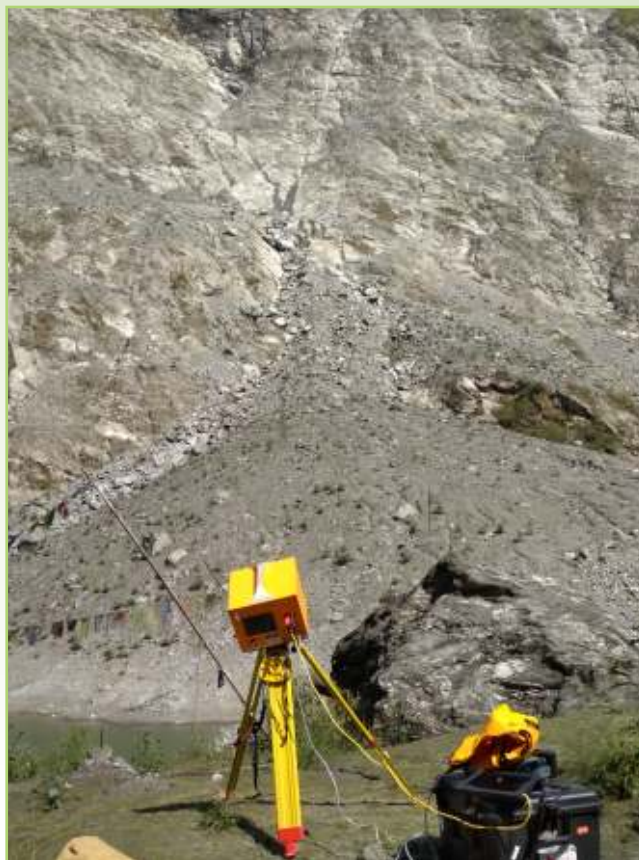
Fig. 57: Terrestrial Laser scanning of the Dzongu landslide that has blocked the tributary of the Teesta river and created a reservoir.
