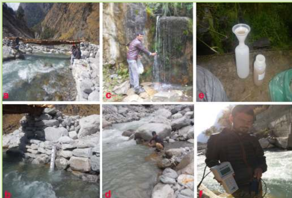
Fig. 52: (a-b) show construction of discharge site, measurement of stage and cross sectional area of the stream. (c-d) display collection of samples for isotopic analysis, (e) sediment filtration process to quantify the SSC and SSL and (f) testing semiautomatic suspended solid analyzer.
