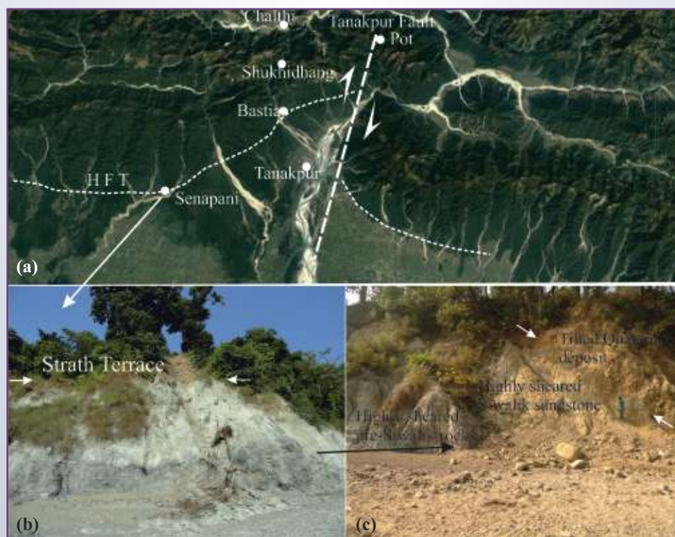
Fig. 25: (a) Google earth image showing displacement of the mountain front as a result of Tanakpur Fault. (b&c) Strath terrace that result from the uplift along the HFT, the bedrock and the overlying Quaternary sediments are tilted moderately towards northwest.
