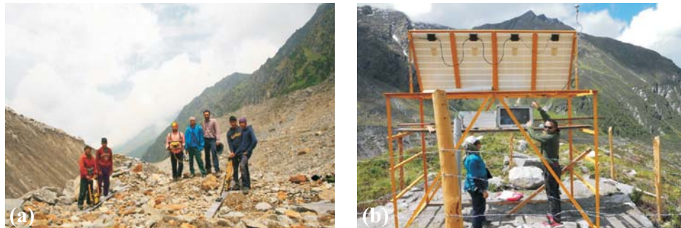
(a) Ground penetrating radar (GPR) survey to measure ice thickness and determine the internal structure of Dokriani Glacier. (b) Data retrieval from Aethalometer installed at Dokriani Glacier for Black carbon measurements
