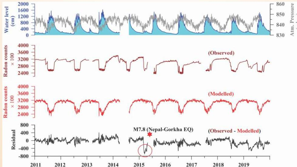
**Fig. 55:** Year-wise (2011-2019) variation of water level and atmospheric pressure (top panel), observed soil radon at 10m depth (second panel), modeled soil radon using water level, and atmospheric pressure (third panel), the variation of residual (bottom panel).
