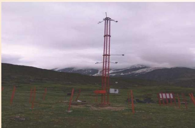
**Fig. 69:** The multi-level sensors installed on a 12 m high mast for detailed land-atmosphere interaction and micrometeorological experimentation at the Pindari glacier site.
