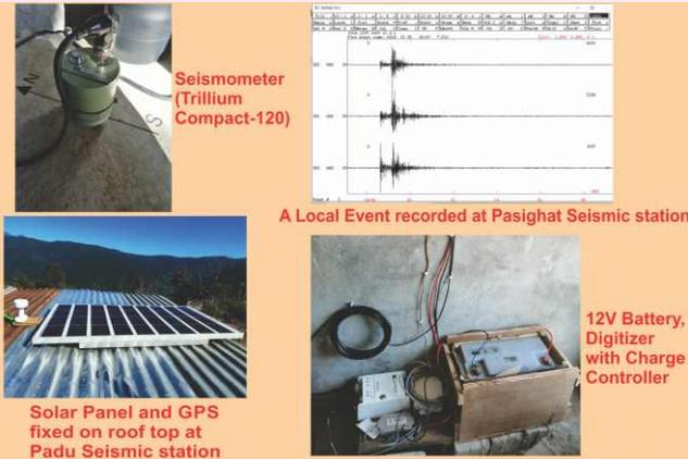
**Fig. 34:** Figure shows the Data Acquisition System at Pasighat Seismic station in Siang Valley of Arunachal Pradesh, and a local earthquake event recorded at Pasighat seismic station.
