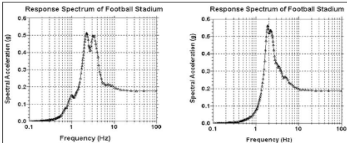
**Fig. 54:** Shows response spectrum of Football stadium located in the center part of the city. The comparison of response spectrum using actual thickness of sediments (140m) (left) and 30m soil column (right) has been shown.
