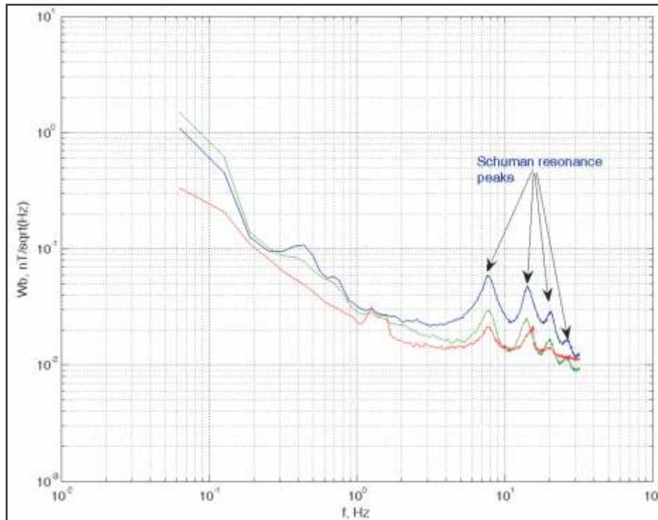
Fig. 66: Schuman Resonance Peaks as observed in Ghuttu.
