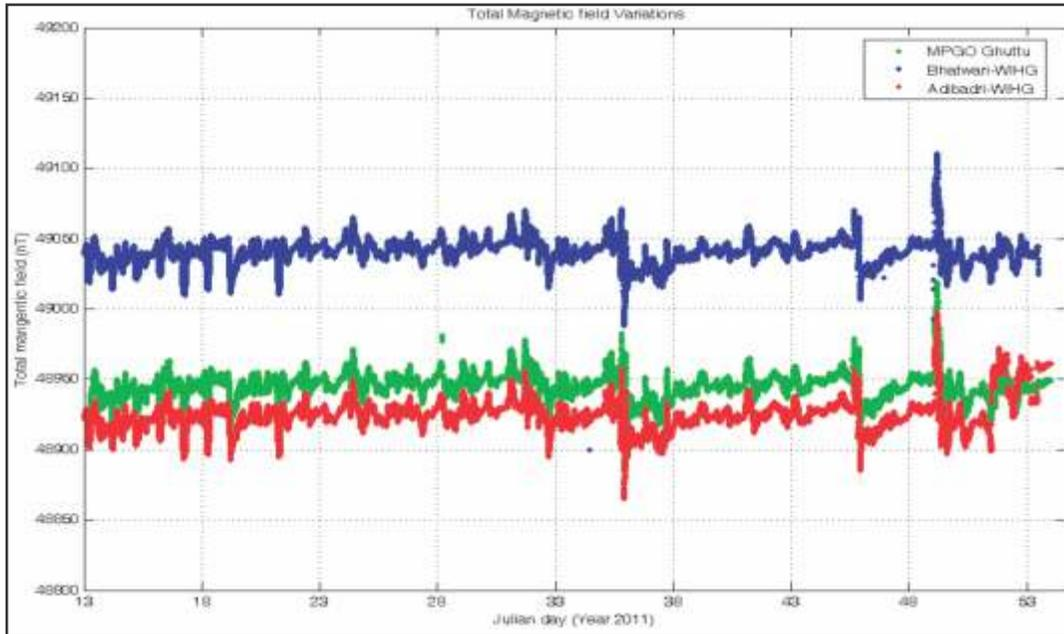
Fig. 64: Total Geomagnetic field variations from Jan 13 -2011 to Feb 22, 2011.
