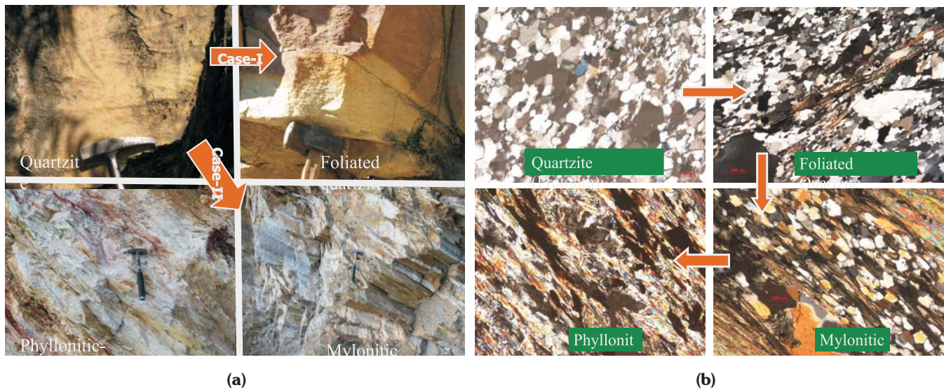
Fig. 2. (a) Macroscopic (b) microscopic features of the protolith quartzite and its progressively deformed foliated, mylonitic and phyllonitic quartzites.
