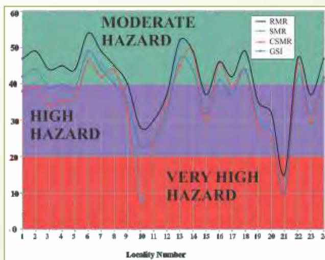
Fig. 53: Different rock mass classifications applied at 24 locations on the bridle path between Janki Chatti and the Yamunotri.
