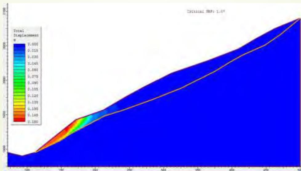
**Fig. 55:** FEM analysis of the Wariya landslide.
