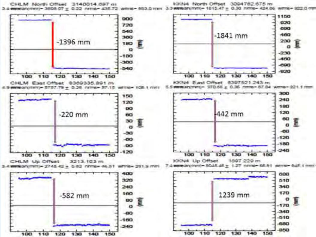
Fig. 9: Near field co-seismic static offsets of 1.8 and 1.4 m are observed respectively in the N-S and E-W components at near stations (distance <100 km from the epicenter) KKN4 and CHLM followed by the Mw 7.8 Gorkha (Nepal) earthquake on 25th April 2015. However, the vertical components show subsidence and uplift respectively at the CHLM and KKN4 stations.
