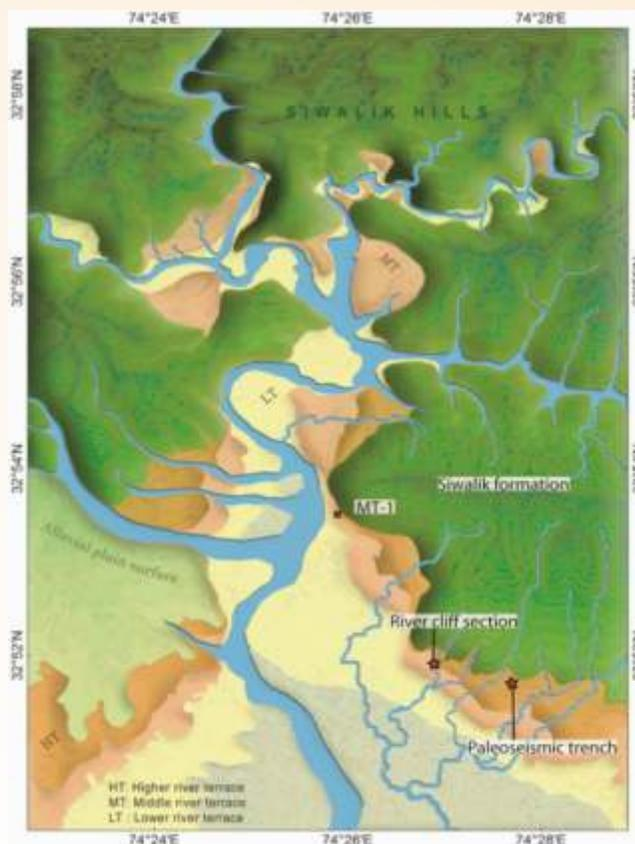
**Fig. 68:** Geomorphic map of River Munwar Tawi showing three levels of terraces and alluvial fans. Paleoseismic trench location and ephemeral tributary cut section cleaned are also shown in the figure. MT-1 shows location of strath terrace along forelimb of SMA.
