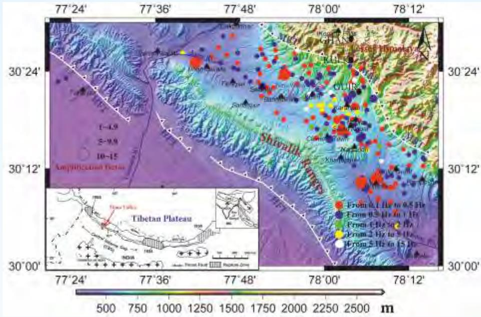
Fig. 8: Spot resonant frequencies and amplification factors of top soil in the Doon valley obtained from seismic ambient noise measurements.
