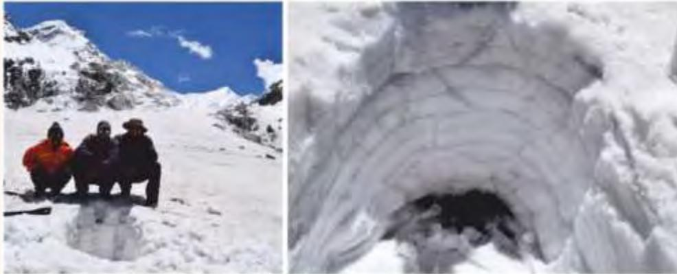
**Fig. 77:** Snow pit (2.6 ft depth) near the accumulation zone of Dokriani glacier for snow density measurements and collection of samples of snow and ice for isotopic and geochemical analysis.
