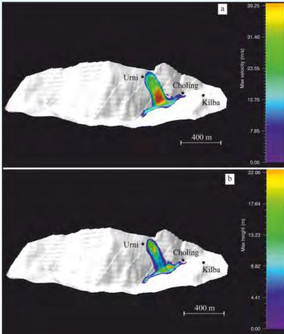
**Fig. 37:** Debris flow run out model of the Urni landslide using rapid mass movement simulation (RAMMS Software).
