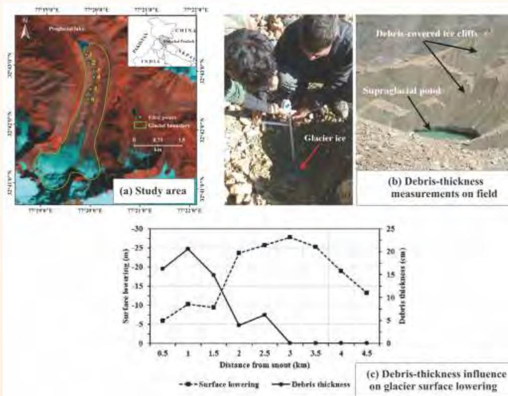
**Fig. 78:** (a) Stake network for ablation measurement, (b) debris-thickness measurement, and (c) influence of debris thickness on surface melting on Panchhi Nala glacier, Bhaga valley, H.P.
