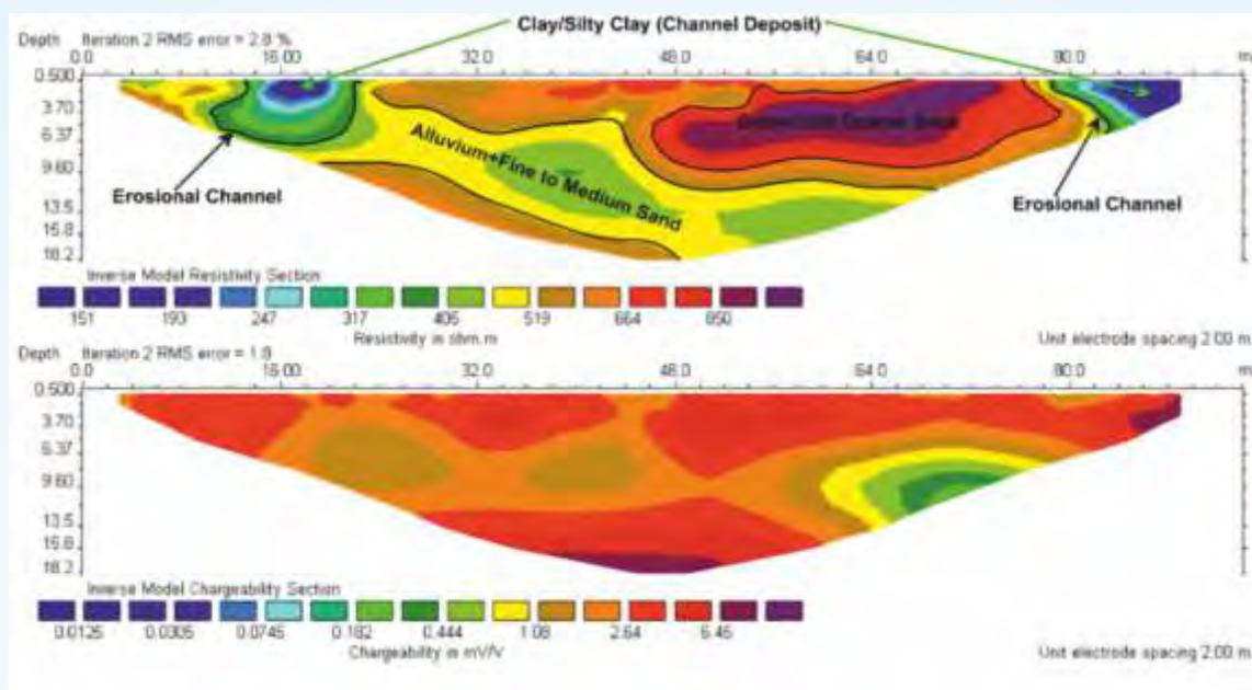
Fig. 32: Inverted 2D section for resistivity and IP-chargeability.
