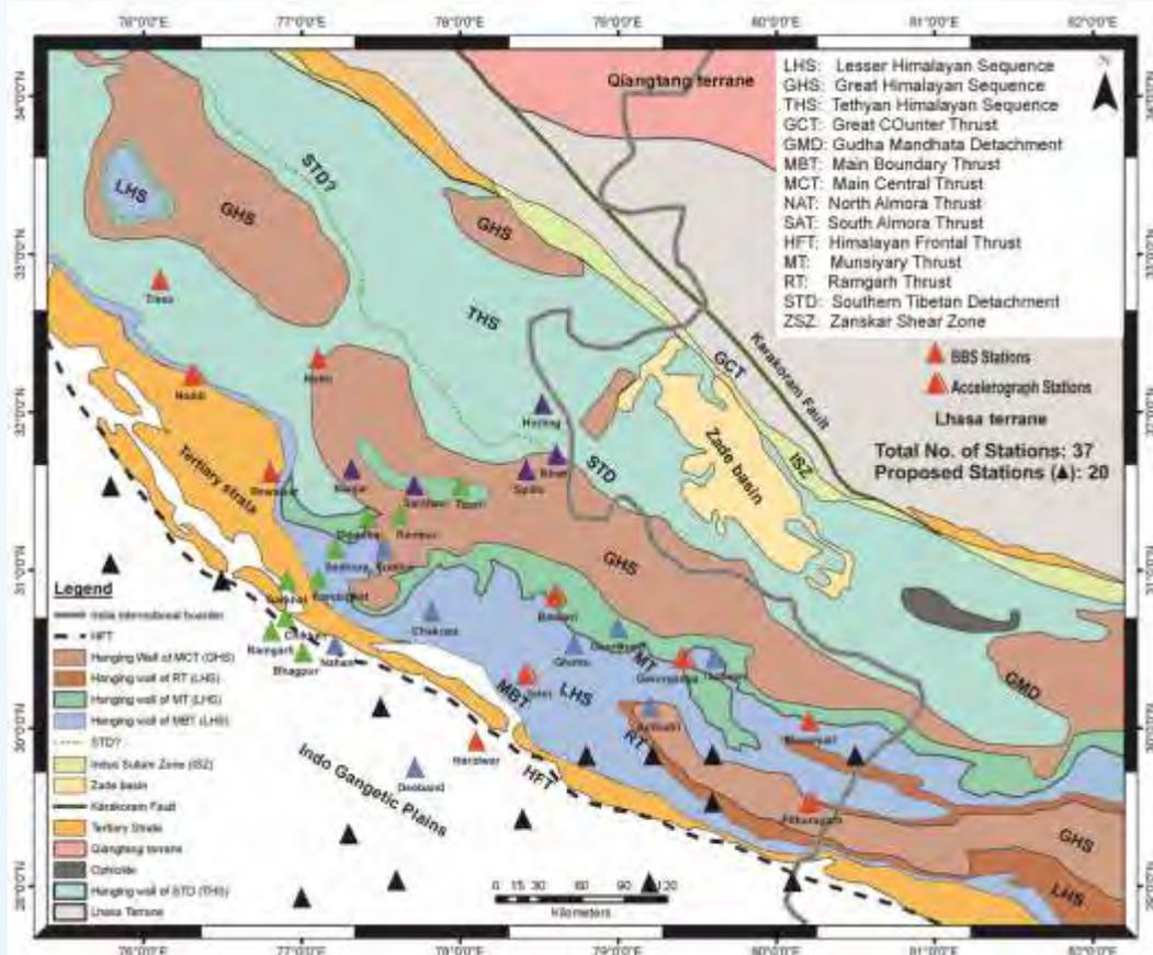
Fig. 21: Broadband seismographs and accelerographs locations are shown with triangles.
