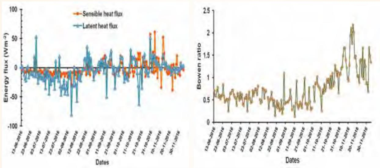
Fig. 73: Daily variation of turbulent heat flux (latent and sensible heat), and seasonal dynamics of Bowen ratio (sensible heat/latent heat) at the Pindari glacier site.
