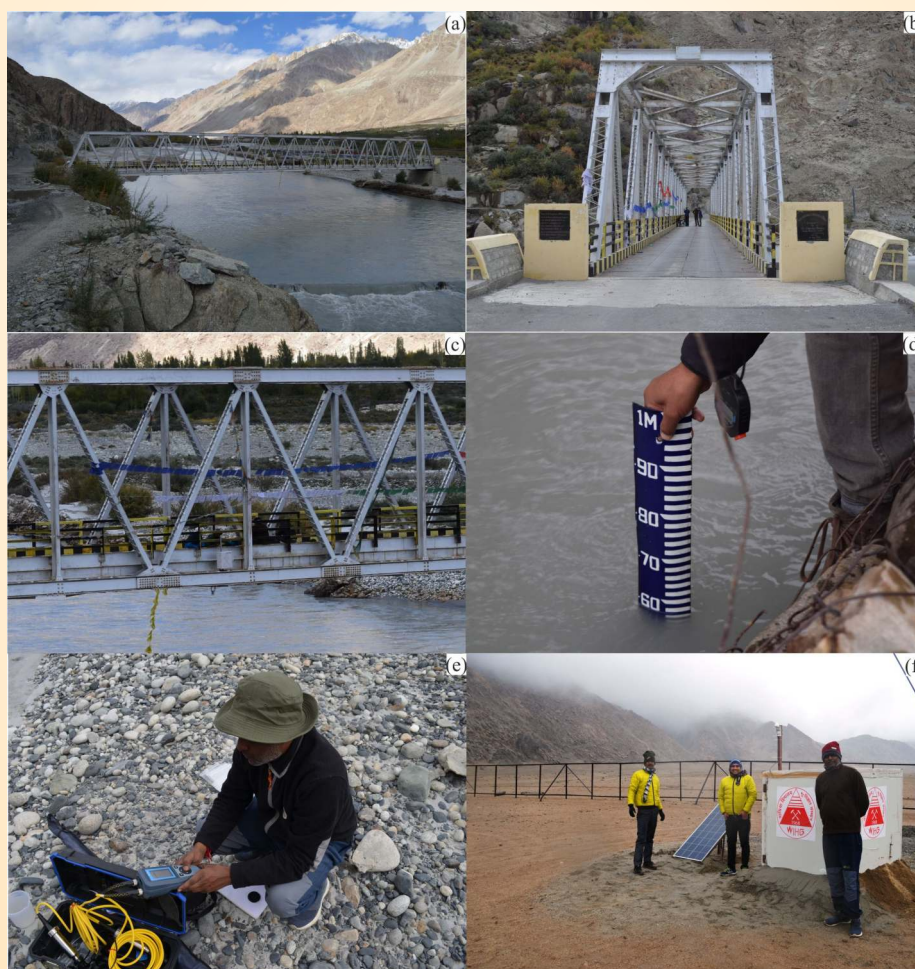
Fig. 63: Location of the metal bridge at Nubra basin near Panamik (a), selection of the suitable site in the middle of the bridge (b) for the installation of AWLR (c) along with observation (manual) of water level (d), physical parameters using multiparameter water quality kit near Panamik (e) and location of installed BBS at University of Ladakh (f).
