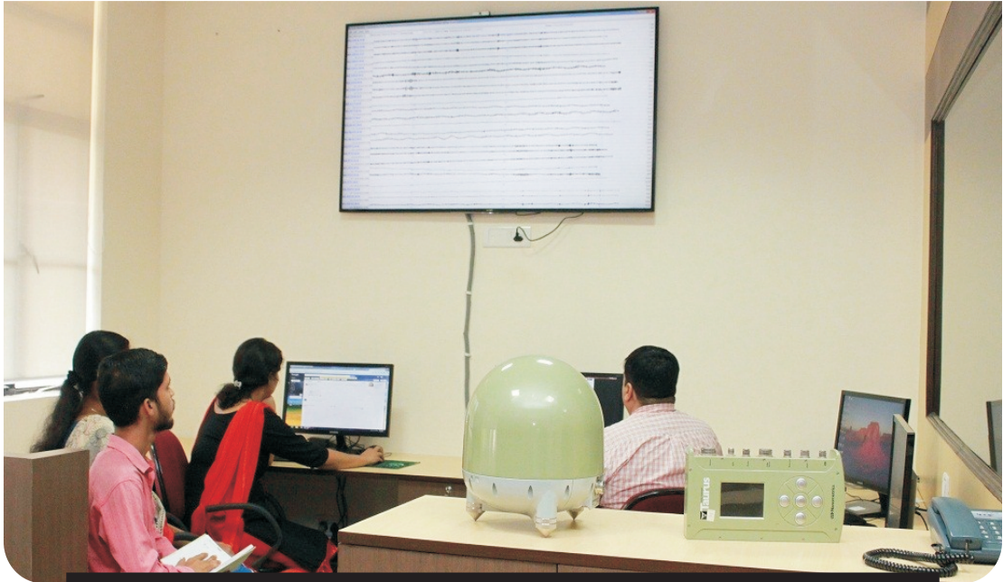
V sat linked Real Time Seismic monitoring lab and display of Trillium 240 Broadband Seismometer and Taurus Digitizer
