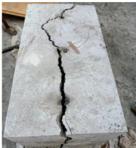
1/2-M 3 M60 Concrete sample cracked in 12h
