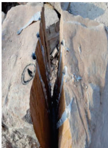
Cracking pattern of CBRI formulation cracked after 15h
