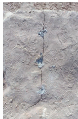
Cracking pattern of CBRI silent cracking mortar.
